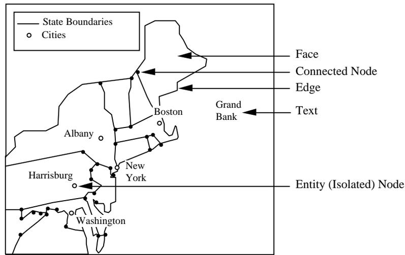
Figure C-5 Geometric and Cartographic Primitives
