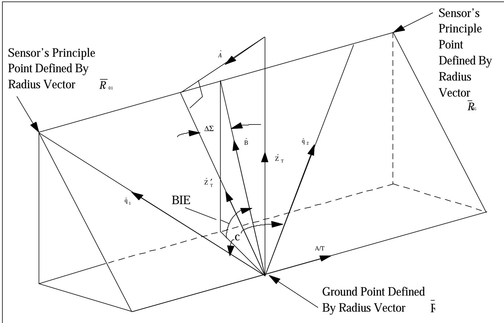
FIGURE 7-1. ILLUSTRATION OF ANGLES INVOLVED IN STEREO IMAGERY
