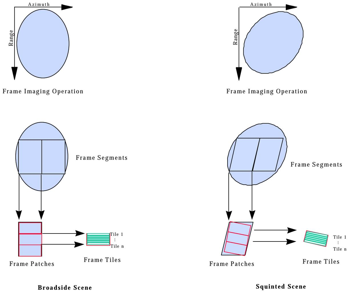
FIGURE 17-2. GENERIC COMPLEX DATA MODEL FOR A FRAME COLLECTION
