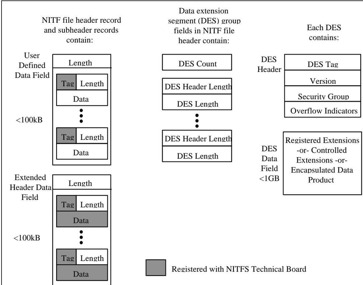
FIGURE 9. Tagged record and data extension segment formats.
