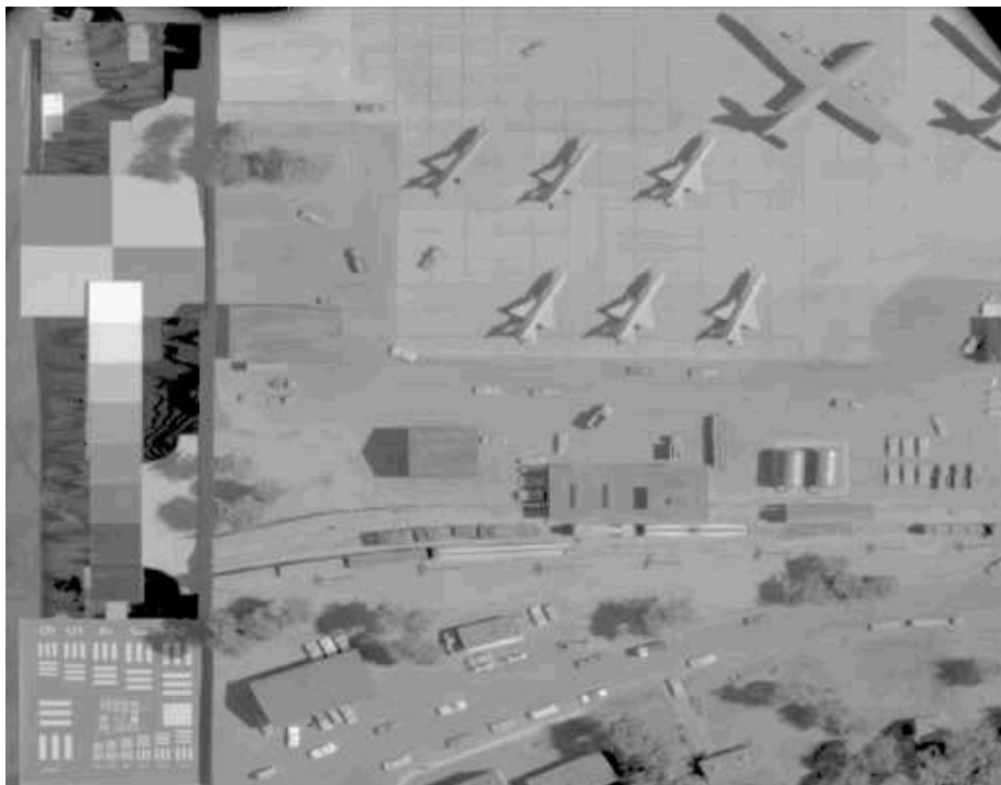
DCT JPEG Q2 Setting – 18,096 Bytes (15 seconds)
