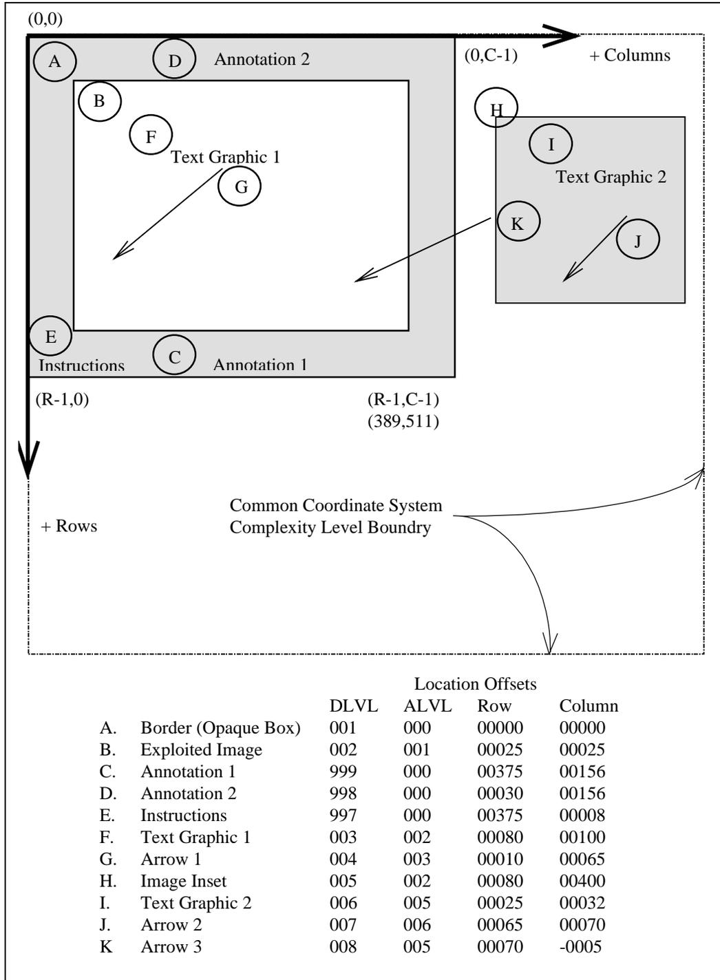
FIGURE 8. NITF Display Level (DLVL) illustration.<sup>†</sup>
