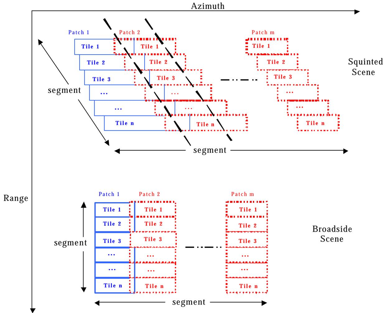
FIGURE 17-3. AIP REPRESENTATION OF A SCAN IMAGE, BROADSIDE AND SQUINTED
