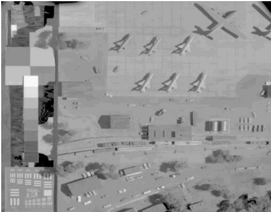
DCT JPEG Q3 Setting – 23,734 Bytes (19 seconds)
