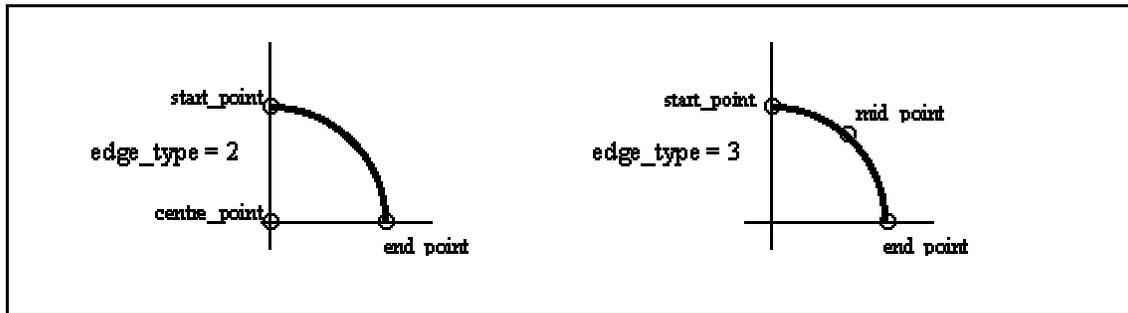
Figure C-18A Geometry for Geometric Circular Arcs
