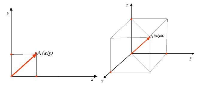
Figure 58: Two and three dimensional coordinate reference systems
