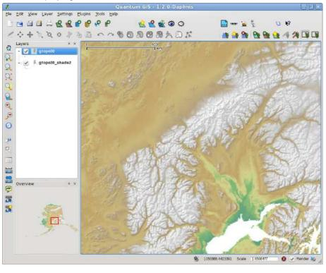
Figure 49: Displaying shaded relief created with the GRASS module r.shaded.relief  $\Delta$
