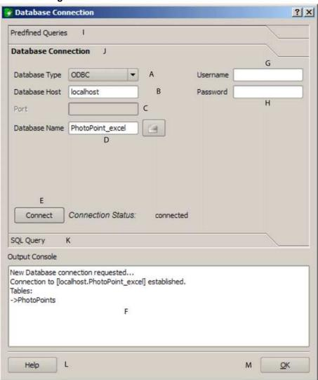
Figure 72: The eVis Database connection window  $\Delta$
