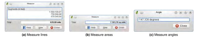
Figure 3.3.: Measure tools in action  $\Delta$
